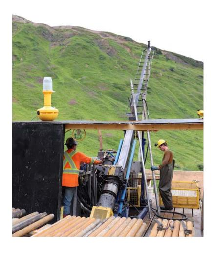
Drillers are pulling core that is being logged by geologists at the core shack
